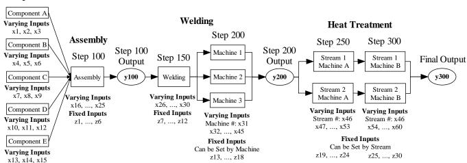
The process produces 1440 parts (camshafts) per day (i.e. one per minute) in three eight hour shifts (midnight to 8am, 8am to 4pm and 4pm to midnight). The plant operates five days per week – there is no production on weekends. At the start it is Monday morning at the start of the first shift.
